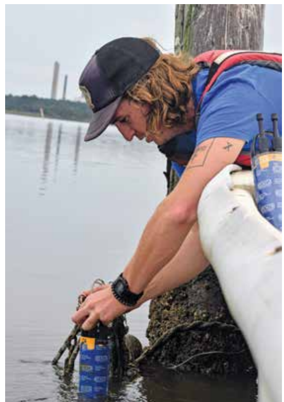
The Center monitors water quality—every 30 minutes, 24 hours a day—using sondes at six sites in the Bays.
