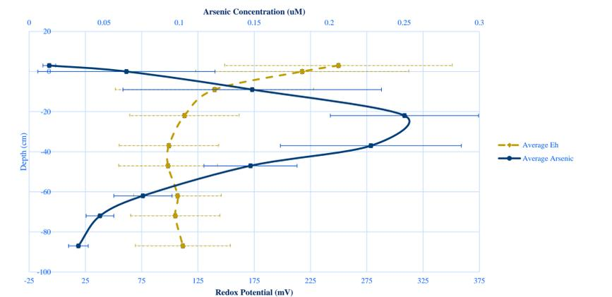
Figure 5: Pore water arsenic and redox potential for near boardwalk peepers
