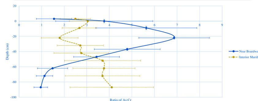
Figure 3: Ratio of As:Cr in different pore water sampling locations at St. Jones
