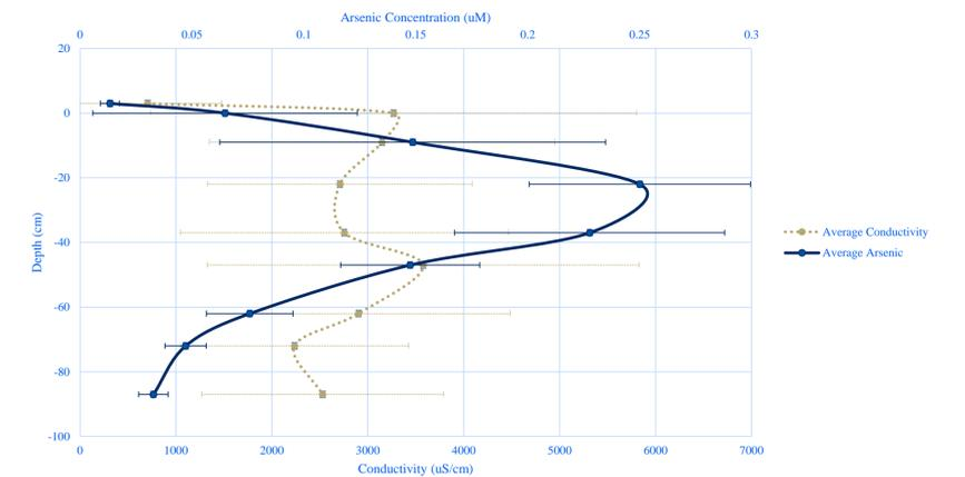
Figure 4: Pore water arsenic and conductivity for near boardwalk peepers
