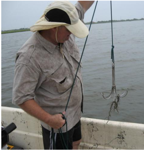
Photo 1: Stainless steel grappling hook used to sample seaweed since 1999 by the author, R. Tyler. Hook was fabricated by William Wireman of Dover, DE.
